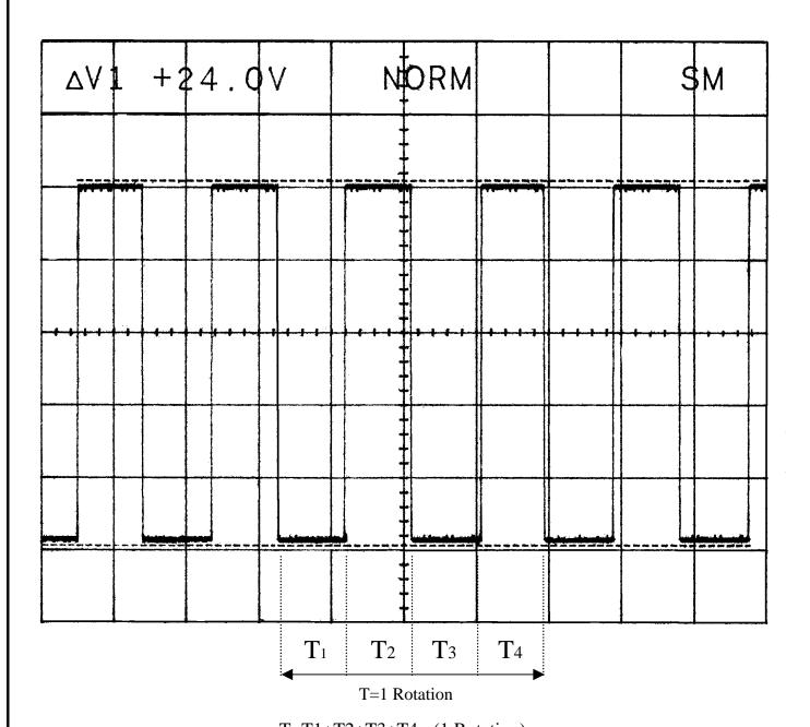
T=T1+T2+T3+T4 = (1 Rotation) $T1=T2=T3=T4= \frac{60}{4 \text{ X rpm}}$
