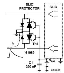
Figure 5. Positive Overvoltage Condition
