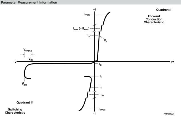
Figure 1. Voltage-Current Characteristic Unless Otherwise Noted, All Voltages are Referenced to the Anode
