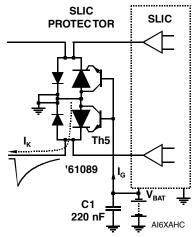
Figure 4. Negative Overvoltage Condition
