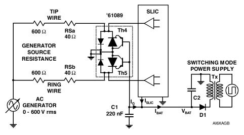
Figure 3. '61089 Buffered Gate Protector
