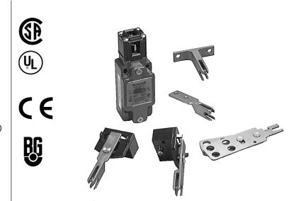
The GK Series is designed specifically for use on machines where key removal brings the machine to an immediate safe condition. It provides enhanced operator safety when added to hinged or sliding guard doors, screens and protective covers on enclosures. The GK Series is especially well suited for large door applications, typically in the automotive plant floor environment. Its heavy duty construction withstands harsh industrial environments where rugged, long-term durability is required.
