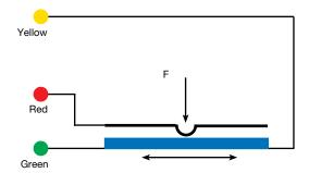
The voltage varies according to the position of the presser on the deformable membrane.
