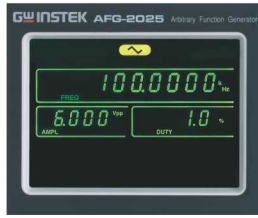
1% Duty Cycle of Square Wave Setting
