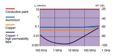
\*SE = Shielding efficiency : equivalent to a  $50\Omega$  load.
