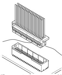
The SHD connector is compact with a mounting height of 6.3mm for top entry type and 5.5mm for side entry type, and a width of 5.0mm for top entry type and 5.1mm for side entry type.
