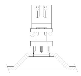
Press the assembly into the mounting hole until the shoulder of the LED is in full contact with the rear of the mounting matrix.
