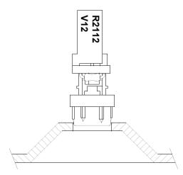
Rotate the product to achieve the required orientation of the connector.
