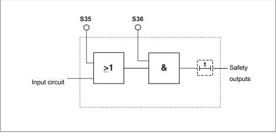
Logic inputs S35 and S36 from the PNOZ e1vp enable additional PNOZelog or PNOZmulti units to be logically AND/OR connected.
