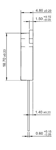
TO3P Pin1 – Base Pin2 – Collector
