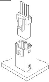
Applicable for waterproof usage. Its waterproof grade is 7 ingress protection of JIS C 0920 (IEC 60529 IPX7).
