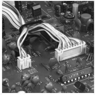
This is a thin, low-profile 2.0mm (.079") pitch connector 7.5mm (.295") in height after mounting and 4.5mm (.177") in width. It is designed to meet the demand for high-density connection of internal wires to printed circuit boards. It is compact, highly reliable and low in cost.
