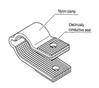
The grounding function is combined with the resin made clamp.
