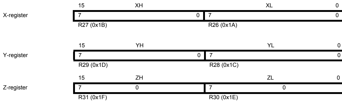
Figure 7-3. The X-, Y-, and Z-registers.
