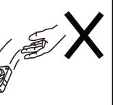
Don't cut the fan or lead wires
