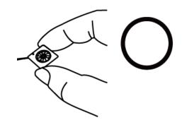
Don't pull fan with lead wires.
