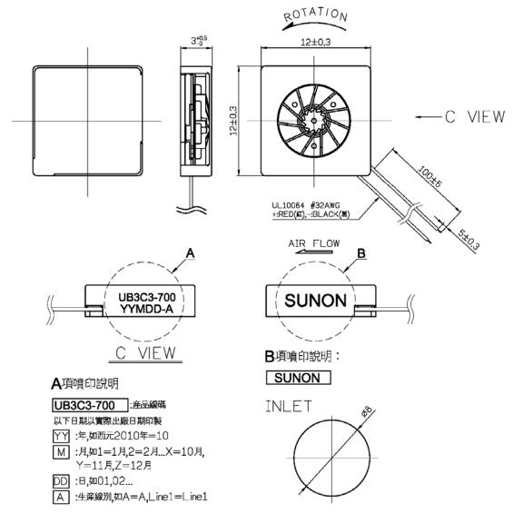
Sunon standard sample exclude the connector. If there is any request for connector, please advise in advance. About recommend connector, SUNON recommend the following models for SUNON Mighty Mini Fan/Blower: 1,(JST) SUR series comector: 02SUR-32S / 03SUR-32S / 04SUR-32S,
