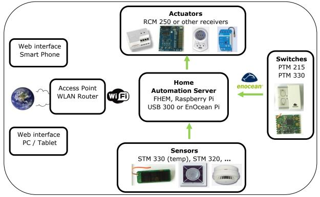
Raspberry Pi with FHEM server acts as home automation server. The server can be used to automate common tasks like switching lamps, scene illuminations or pulling blinds, measure and visualize power consumption, temperature and humidity.
