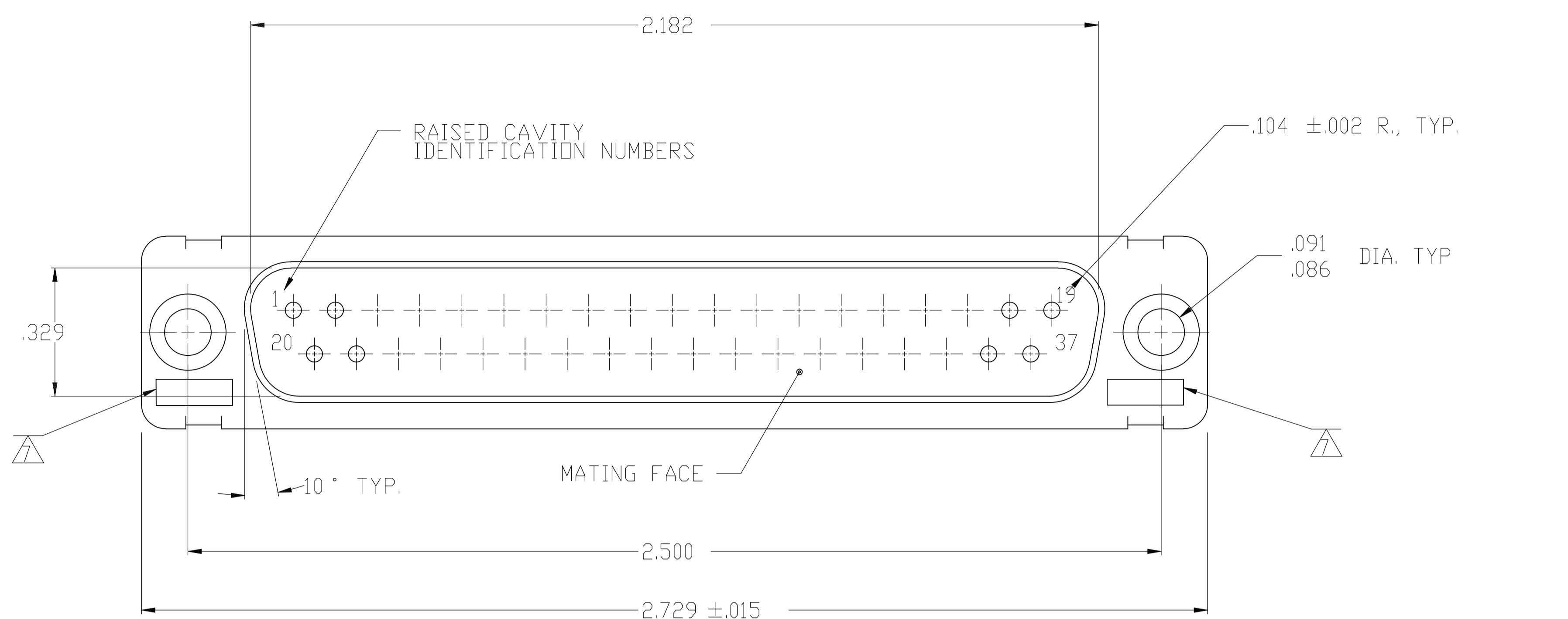
1. THIS PLUG IS DESIGNED TO CONFORM TO THE LATEST ISSUE OF MIL-C-24308
