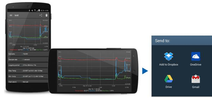
View logged temperature, humidity readings and calculated dew point, minimum and maximum values, and alarm breaches. Use zooming and panning features to view critical data with ease.
