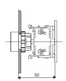
Dimensions of minimum space requirements (according to EN 50007 and IEC337-2C). Take to consideration the field of traverse of swing knobs (27mm) and the diameter of mushroom heads.
