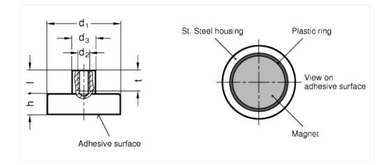
technical informations Specification Disc shaped, with female thread Housing / threaded bush, stainless steel
