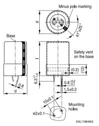
Minus pole marking Base Safety vent on the base 3 (0.2)4.5-1.4 0.8+0.2 0.8 1.5±0.2 d 1020 ø2±0.1 Mounting holes 3.3±0 ø2.5 min. KAL1177-Y-E
