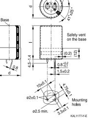
Snap-in terminals, length (6.3 + 1/-1.4) mm. Also available in a shorter version with a length of (4.5 - 1.4) mm. PET insulation cap is positioned under the insulation sleeve.
