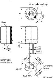
Snap-in capacitors are also available with 3 terminals (length (4.5 - 1) mm). PET insulation is marked with label "PET" on the sleeve.
