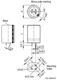
Snap-in capacitors are also available with 3 terminals (length (4.5-1) mm). PET insulation is marked with label "PET" on the sleeve. Safety vent on the base or on the case wall.
