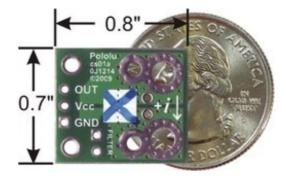
This current sensor is a carrier board or breakout board for Allegro's ACS714LLCTR-05B-T Hall effect-based linear current sensor; we therefore recommend careful reading of the ACS714 datasheet (678k pdf) before using this product. The sensor operates at 5 V and has an output sensitivity of 185 mV/A. The board ships fully populated with its SMD components, including the ACS714, as shown in the product picture. The following list details some of the sensor's key features:
