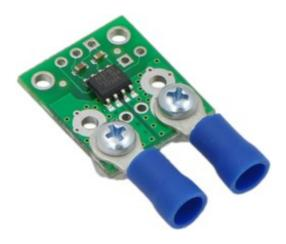
ACS715 current sensor carrier with solderless ring terminal connectors (not included).
