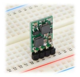
This regulator is also available with a fixed 5 V output or a fixed 9 V output.
