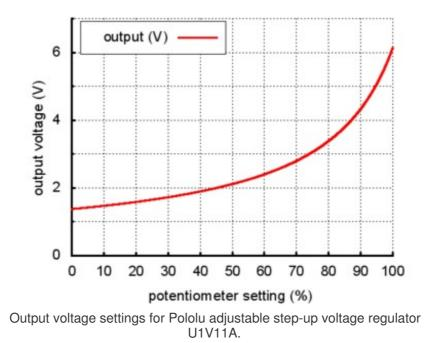
Please note that the output voltage can be set below 2 V at the low end of the potentiometer's range and above 5.25 V at the high end. While this should not harm the regulator, it might not work reliably or its output could become unstable when the output voltage is not within the recommended 2 V to 5.25 V range. In addition, the potentiometer has no physical end stops, which means that the wiper can be turned 360 degrees and into an invalid region in which the output voltage is unstable.
