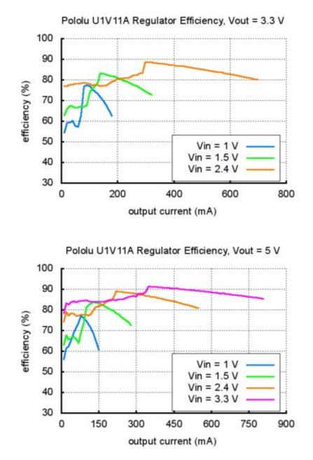
The maximum achievable output current is approximately proportional to the ratio of the input voltage to the output voltage. If the input current exceeds the switch current limit (typically somewhere between 1.2 and 1.5 A), the output voltage will begin to drop. Additionally, the maximum output current can depend on other factors, including the ambient temperature, air flow, and heat sinking.
