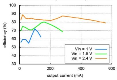
The maximum achievable output current is approximately proportional to the ratio of the input voltage to the output voltage. If the input current exceeds the switch current limit (typically somewhere between 1.2 and 1.5 A), the output voltage will begin to drop. Additionally, the maximum output current can depend on other factors, including the ambient temperature, air flow, and heat sinking.
