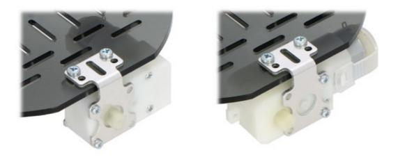
These brackets also work with the Solarbotics plastic gearmotors (GM2, GM3, GM8, and GM9), although different length mounting screws might be required.
