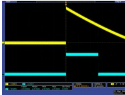
QTR-1RC output (yellow) when 1/8" above a black line and microcontroller timing of that output (blue).
