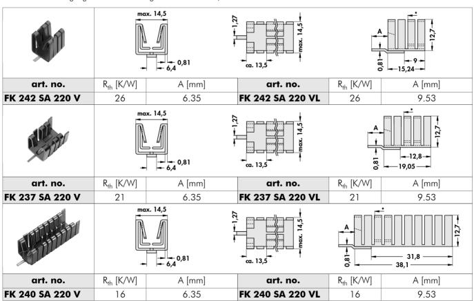
\* = touch in edge of transistor material: aluminium surface treatment: black anodised
