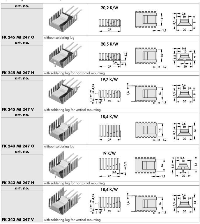
material: copper (Cu) material thickness: 0.6 mm surface treatment: solderable
