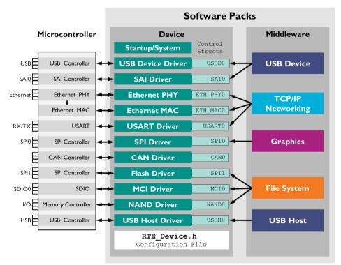
Middleware components usually have various configuration files that connect to these drivers. For most devices, the *RTE\_Device.h* file configures the drivers to the actual pin connection of the microcontroller device.
