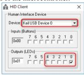
To test the functionality of the USB HID device run the *HIDClient.exe* utility and follow these steps:
