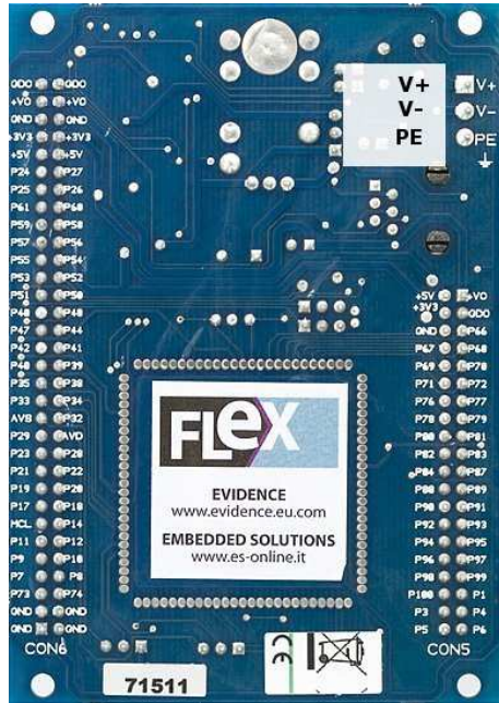
Figure 3.8: Rear view of the FLEX Light version, with highlighted power supply pins (original photo courtesy of Sparkfun).
