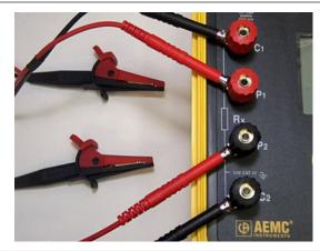
For the probes with Red/Blk and Red/Blk leads and Red DOT located on the probe tip: Connect them as shown here.
