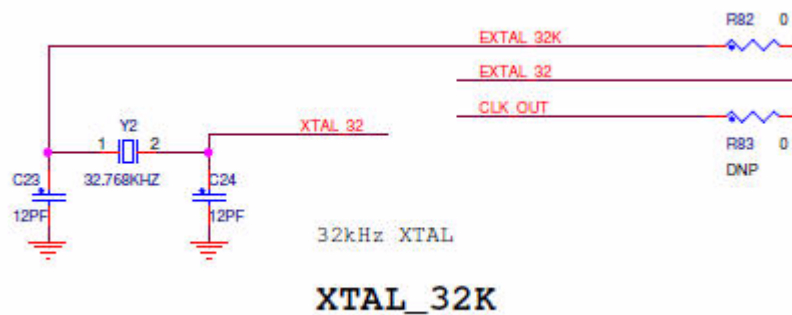
Figure 3-6. TWR-KW24D512 32.768 kHz Optional Oscillator Circuit
