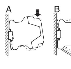
The assignment of the connection terminal blocks is shown in the block diagram. The module can be snapped onto all 35 mm DIN rails according to EN 60715.
