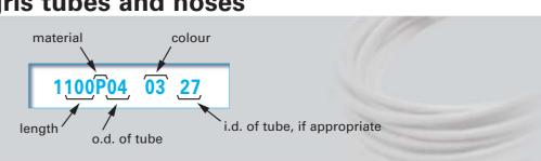
tube o.d.: corresponds to the outside diameter of the tube
