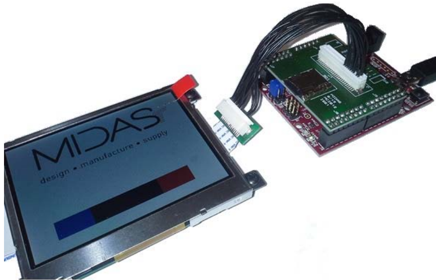
Figure 1. Example of the MCIB-12 Board used in conjunction with both the UNO32 and MPBV5 boards to power one of our range of TFT Displays. It also uses the SDHR-50V-S-B connector and MCCBL-SHDR-SHDR-100 cables which can all be seen in the picture above.
