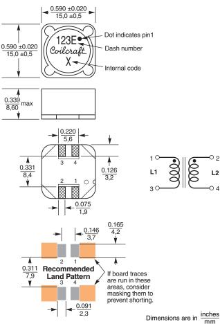
Excellent coupling coefficient (k  $\geq$  0.98) and 500 Vrms isolation makes the MSD1583 series of coupled inductors ideal for use in a variety of circuits including flyback, multi-output buck, SEPIC and Zeta. These parts provide high inductance, high efficiency and excellent current handling. In SEPIC topologies, the required inductance for each winding is half the value needed for two separate inductors, allowing selection of a part with lower DCR and higher current handling.
