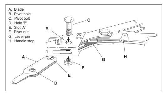
The diagram above gives a view of the nibbler blade assembly. Firstly ensure that the handle stop is released as shown. Slide the blade into the frame locating slot A around the lever pin and align hole B with the pivot hole. Pass the pivot bolt through and screw it into the frame. Lock the bolt with the pivot nut.
