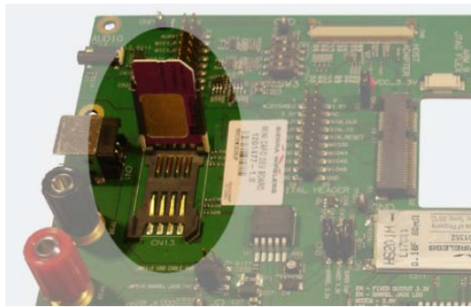
Figure 2-3: Inserting a SIM into the open cover
