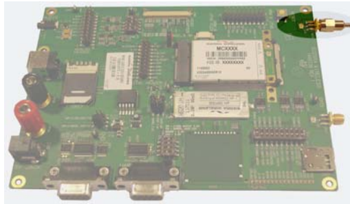
Figure 2-8: Connecting the antenna adapter
