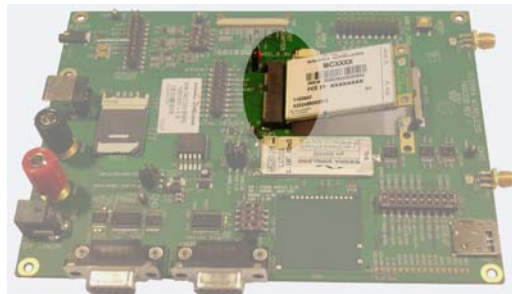
Figure 2-6: Inserting a Mini Card
