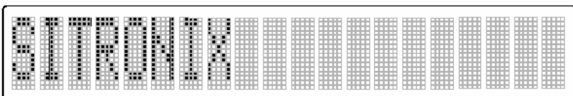
1 line mode with double height font (DH=1/N=0)
