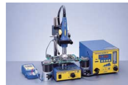
Setting example HAKKO FR-803B, HAKKO FR-820, Rework Fixture, Omnivise
