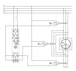
S<sub>6</sub> - main connector S<sub>△</sub> - connector of system "DELTA" S<sub>→</sub> - connector of system "STAR"
