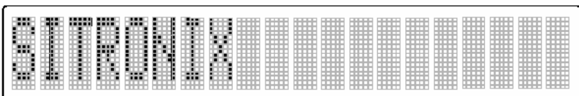
1 line mode with double height font (DH=1/N=0)
