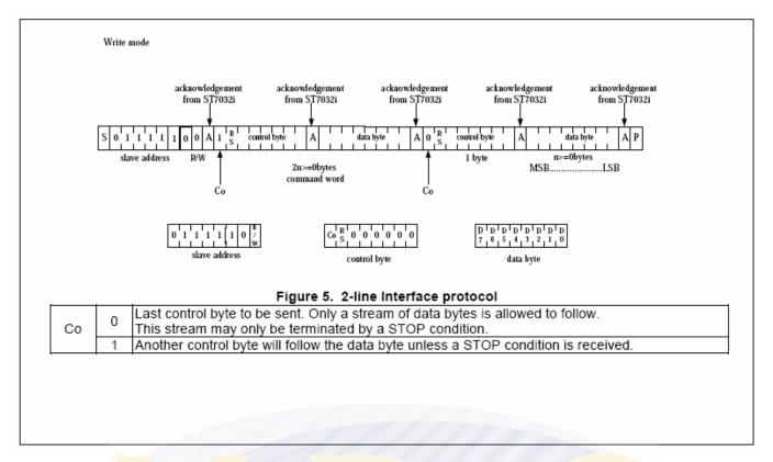
During write operation, two 8-bit registers are used. One is data register (DR), the other is instruction register
