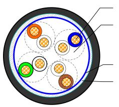
Conductor (26AWG/7 – 7x0.16mm Stranded Tinned Copper)
