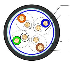
Conductor (26AWG/19 - 19x0.1mm Stranded Tinned Cu)
