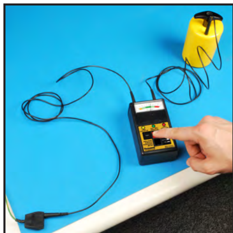
Figure 3. Using the test leads and one 5 pound electrode to measure Rg
