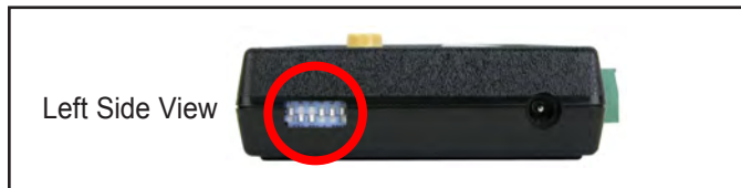
Figure 2. Locating the DIP switch on the SmartLog V4™ Tester, Dual Independent Tester and Combo Tester X3
