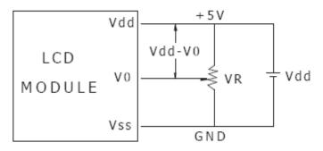
Vdd-V0: LCD Driving Voltage
