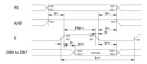
NOTE: \*VOL1 is assumed to be 0.8V at 2 MHZ operation.
